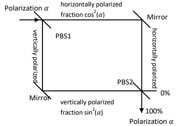
**Figure 3:** Beam paths at a Mach-Zehnder Interferometer (MZI) with polarizing beam splitters without interference
