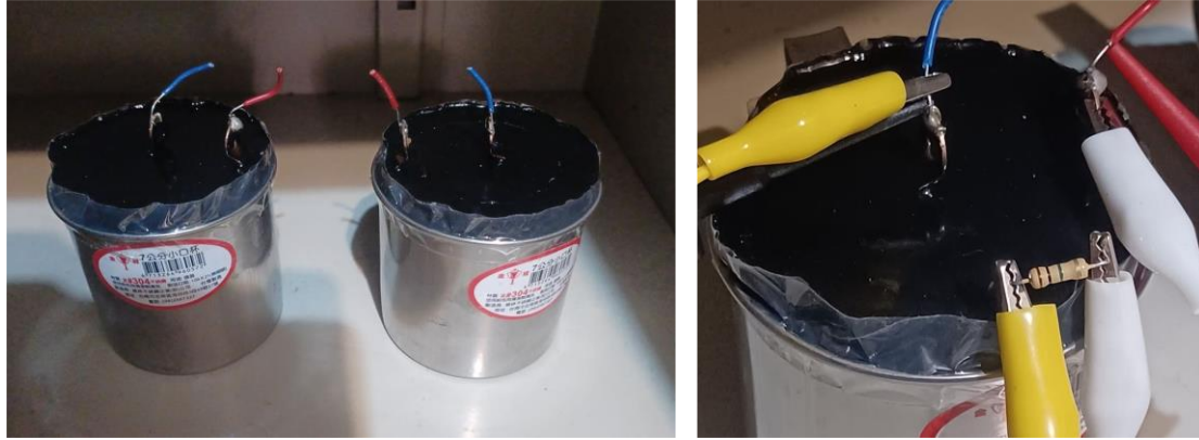
Fig. 10. Selected images of the gravity battery during the static measurement process.
