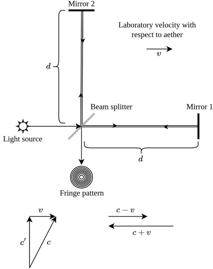
Figure 3: Experimental setup for the Michelson-Morley interferometer.
