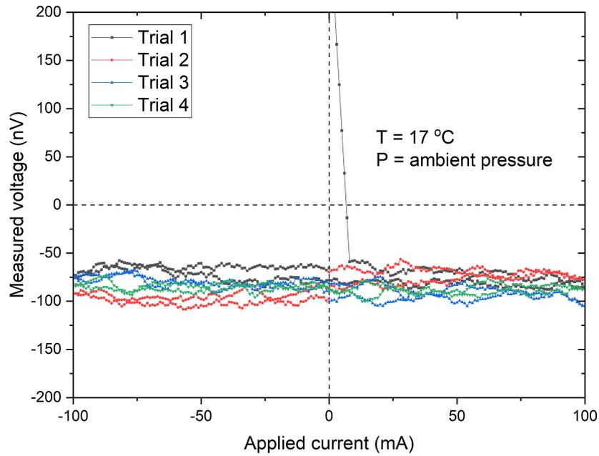
Fig. 4. Measured voltages for applied current ranging from -100 mA to 100 mA (sample #6).
