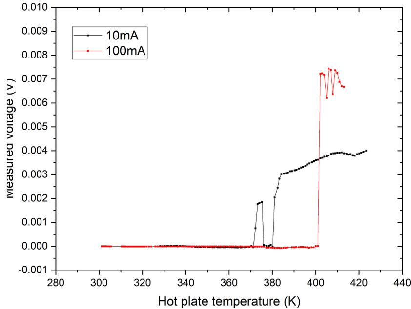
Fig. 9. Temperature dependence and phase transition of sample#8 for applied current of 10 and 100 mA.
