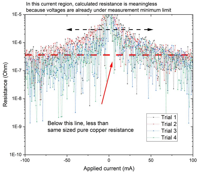
Fig. 3. Resistances of sample #5 for applied current ranging from -100 mA to 100 mA (data from Fig. 2).
