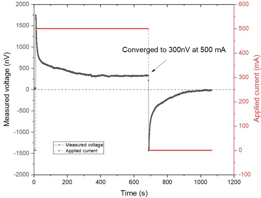
Fig. 11. Voltage decay phenomenon of sample #5 for applied current of 500 mA.
