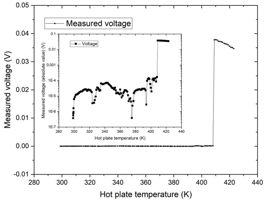
Fig. 7. Temperature dependence and phase transition of sample#5 for applied current of  $1 \mu\text{A}$ .
