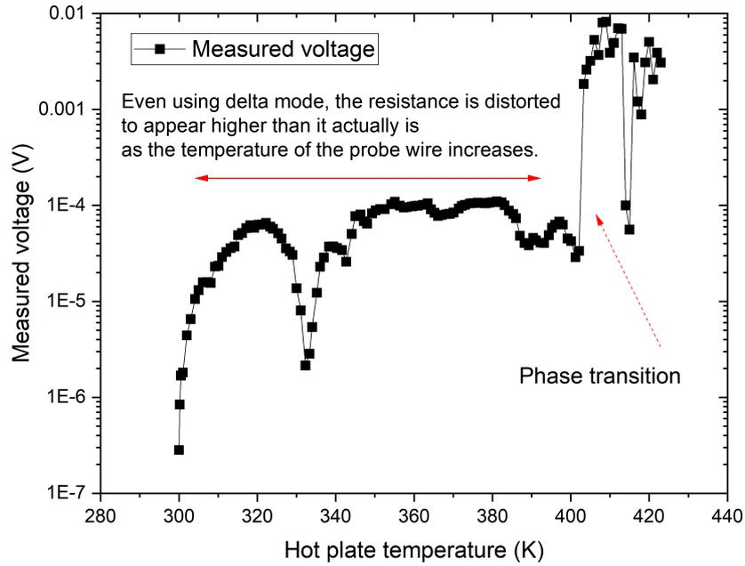
Fig. 10. Temperature dependence and phase transition of sample#5 for applied current of 10 mA, delta mode.
