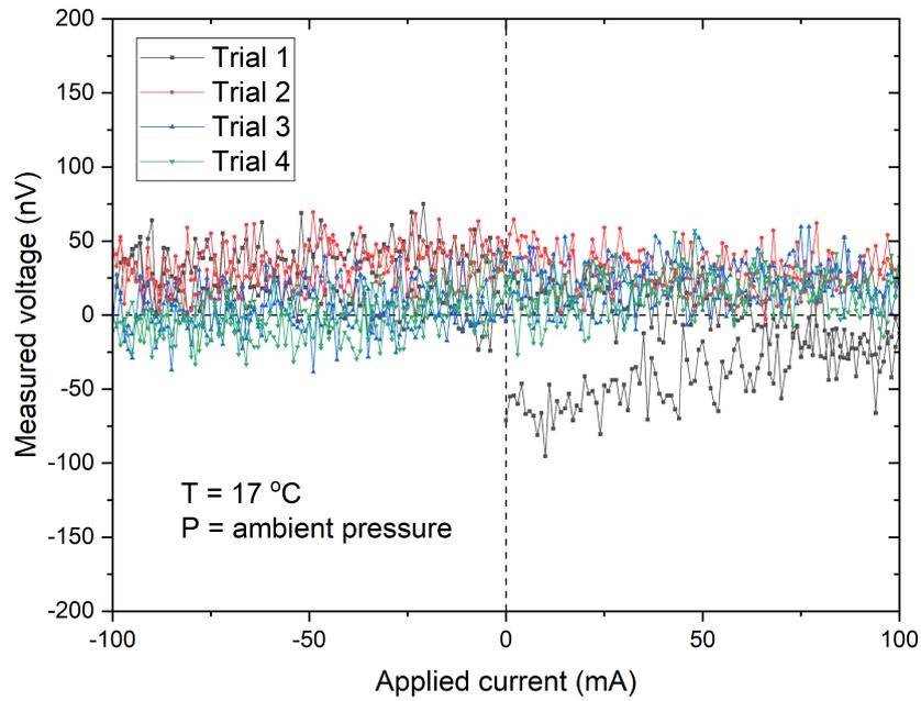
Fig. 2. Measured voltages for applied current ranging from -100 mA to 100 mA (sample #5), (newly measured data).
