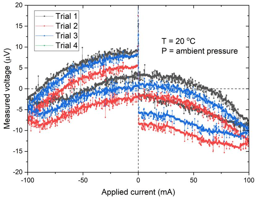
Fig. 5. Measured voltages for applied current ranging from -100 mA to 100 mA (sample #8).
