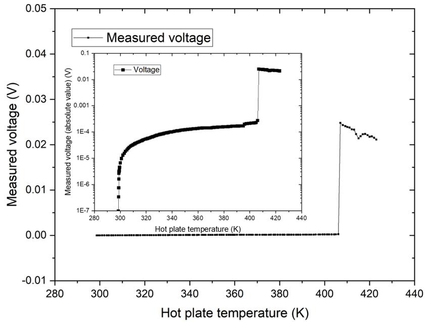
Fig. 8. Temperature dependence and phase transition of sample#8 for applied current of  $1 \mu\text{A}$ .
