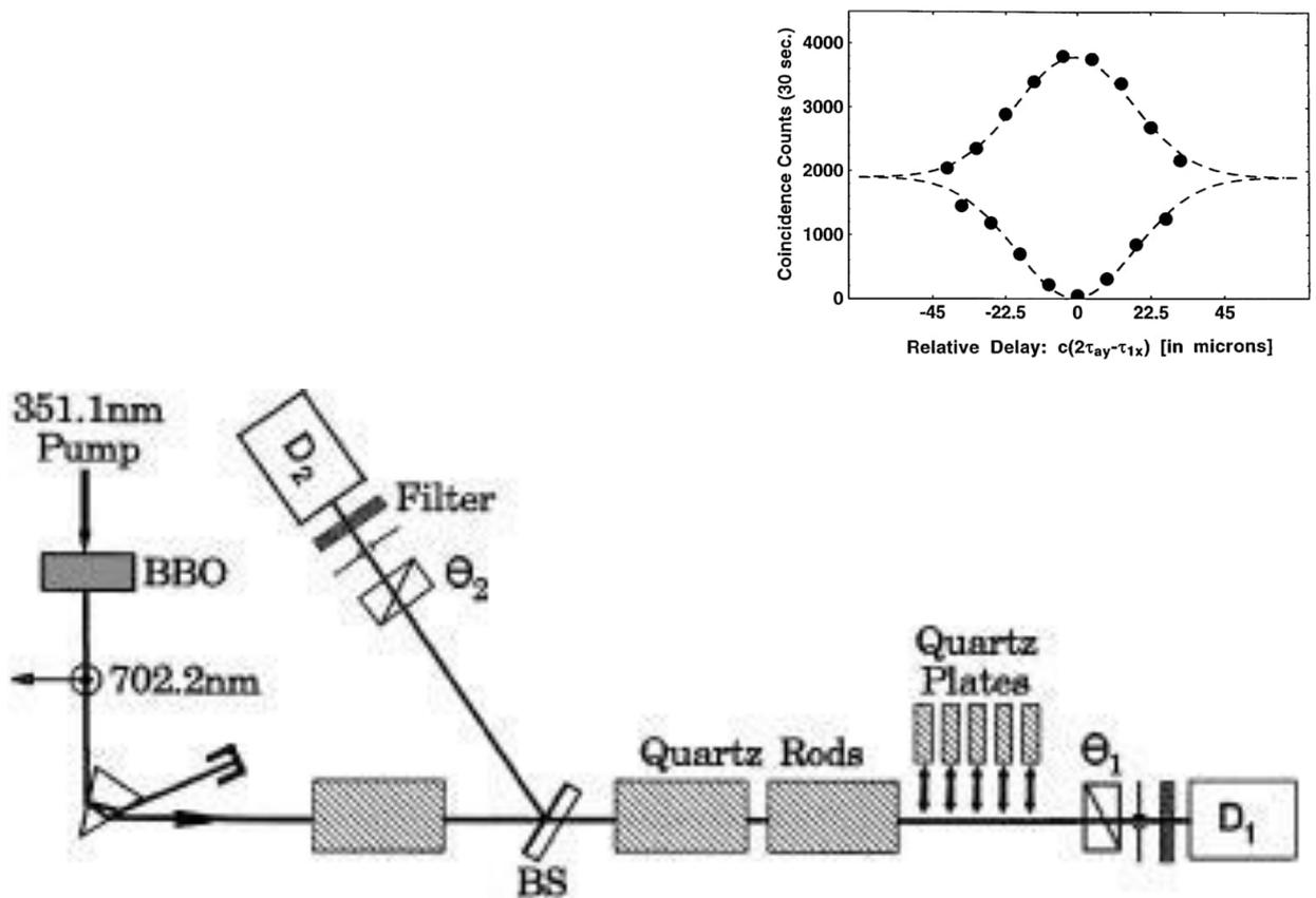
Fig. 1 Scheme of the experiment and its result [9].
