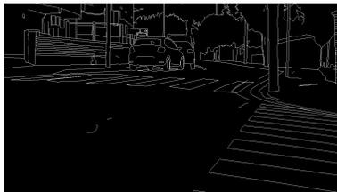
Figure 2. RGB\_003: Edge detected with classical computer & methods
