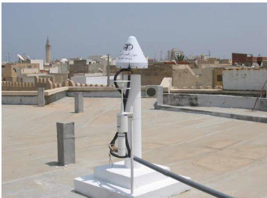
FIGURE 3.3 – Station GPS Permanente de Monastir
