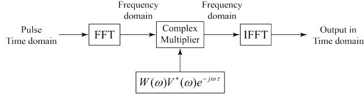
Fig. 1 The diagram of LFM pulse compression using the spectral window
