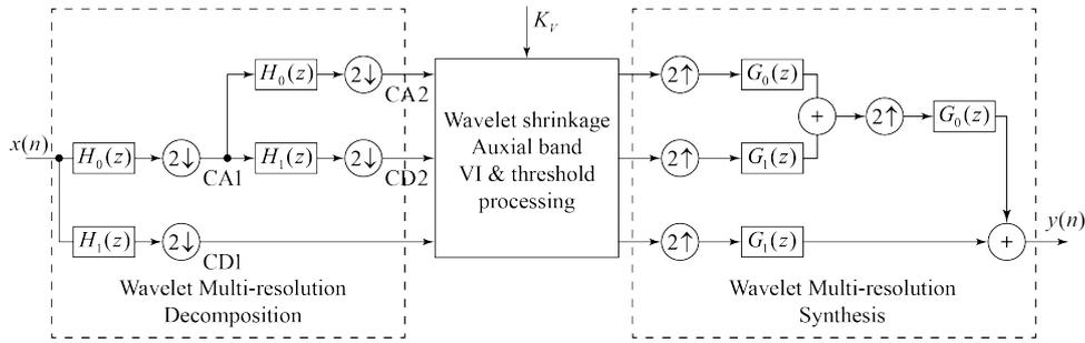
Fig. 3 Diagram of the VI-wavelet threshold processing for the sidelobe reduction
