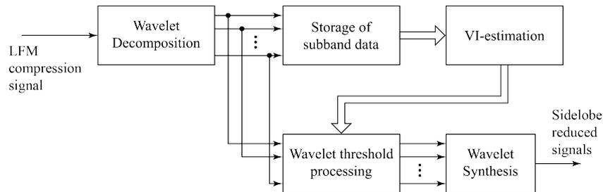
Fig. 2 VI-wavelet shrinkage adaptive processing diagram
