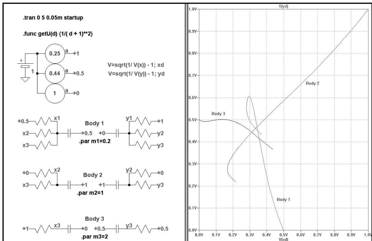
Body 1 wants to fly from  $x=+0.5$ ,  $y=+0$  to  $x=+0.5$ ,  $y=+1$ . Body 2 from  $x=+1$ ,  $y=+1$  to  $x=+0$ ,  $y=+0$ . Body 3 from  $x=+0$ ,  $y=+0.5$  to  $x=+1$ ,  $y=+0.5$ . All three bodies gravitate with each other.
