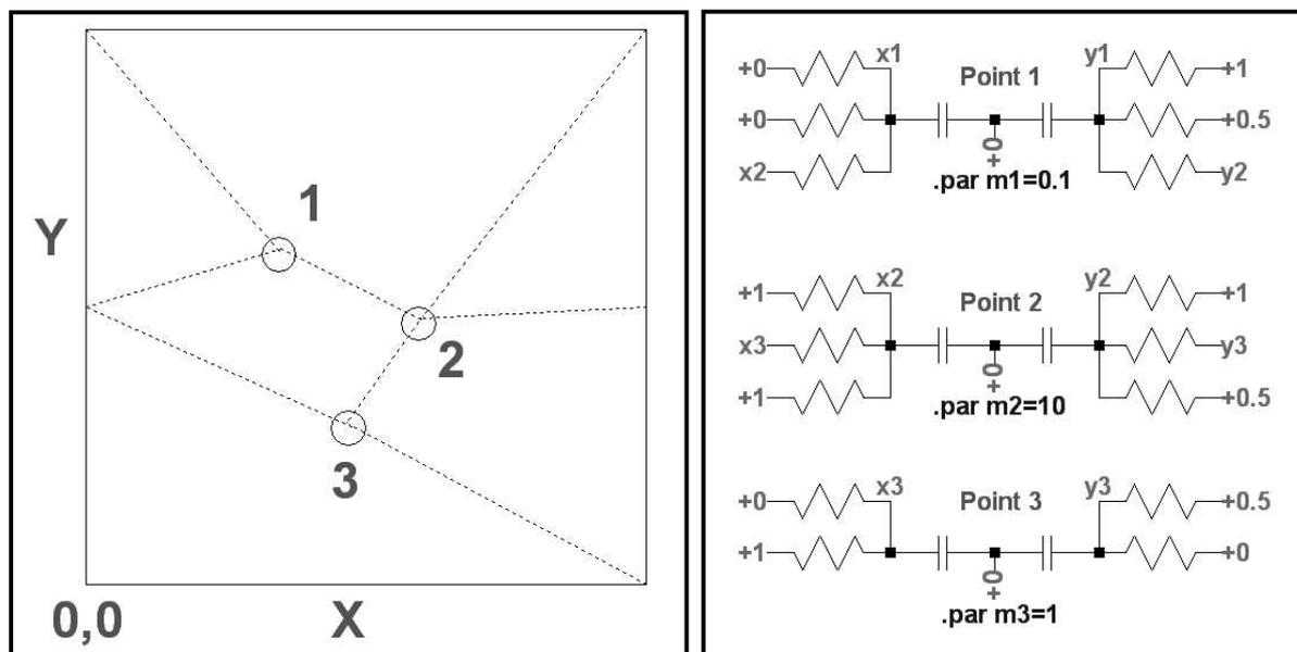
Starting from point 1 ( $x_1/y_1$ ), three "rubbers" are programmed with two resistors each:
