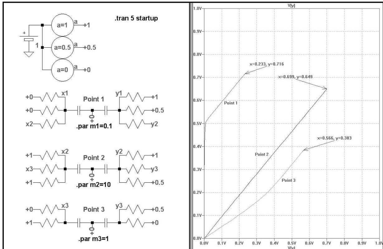
Since the capacitors have a time-delaying effect, a dynamic system is created. The positions of the three points in the course of the calculation are plotted on the right. The three marked end points of the three nuts is the optimal solution of the task.
