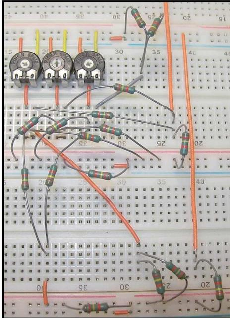
The \$2 setup consists of the voltage source that powers the three 10k trimmers and the 16 resistors. The capacitors were omitted to achieve the maximum computing speed.
