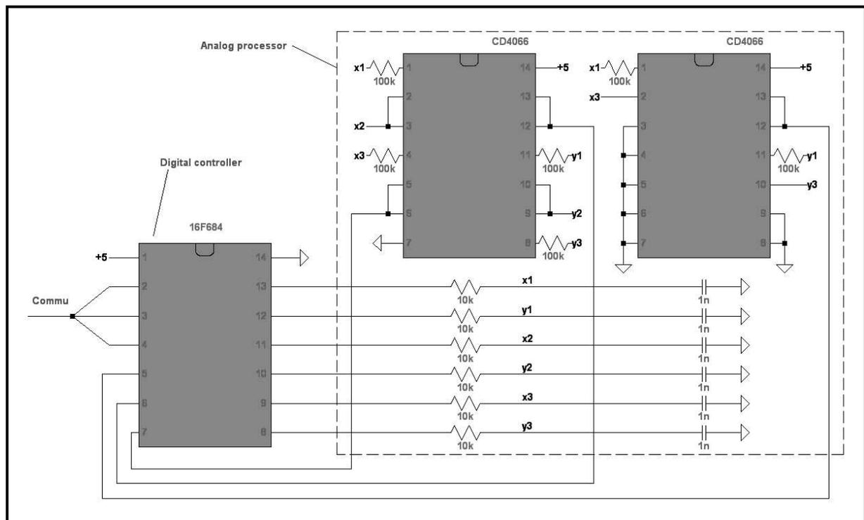
The three trimmers are replaced by six digitally generated voltages that act directly on x1, y1, x2, y2, x3 and y3. The cross-connections are realized with three double-pole analog switches. By PWM-clocking these switches, the effect of the cross-connections can be varied from 0% to 100%.
