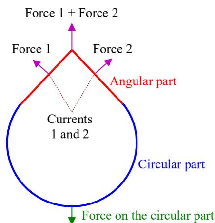
Figure 11 Coil with angular and circular parts
