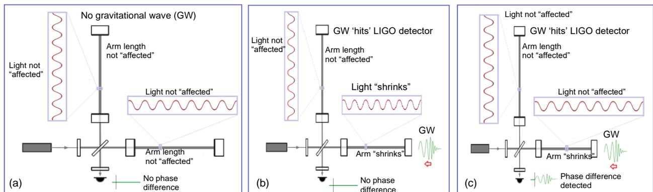
**Fig 2:** Three LIGO detector cases: a) No gravitational wave “hits” the detector. b) Gravitational wave “shrinks” the arm length and “shrinks” the light fields (no phase difference). c) Gravitational wave “shrinks” the arm length and light is not affected (phase difference detected).
