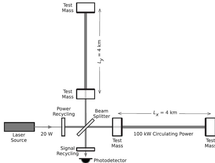
**Fig 1:** The LIGO detector: A modified Michelson interferometer.
