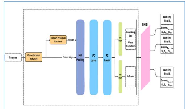
Figure 3: Architecture of Faster RCNN
