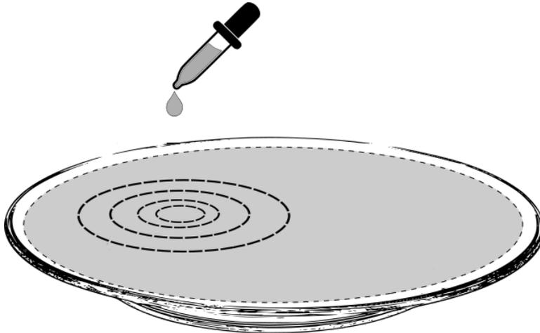
Figure 4: The Water Wave experiment may be performed using a circular platter and any suitable means to initiate an isotropic wave on the surface of the water.
