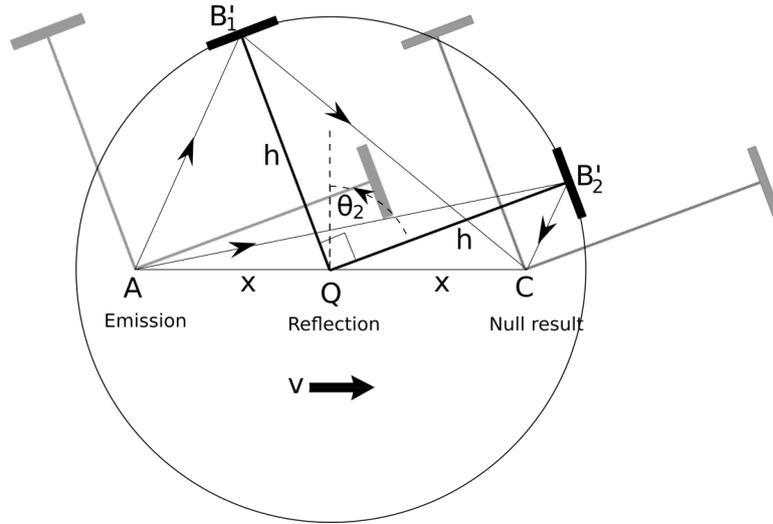
Figure 3: Geometry of the Michelson-Morley experiment depicting the general case  $x \neq 0$ . Equivalent to our thought experiment and identical to fig. 1, we find  $AB_1' + B_1'C \neq AB_2' + B_2'C$  but yet we agree that the outcome is a null result at point  $C$ .
