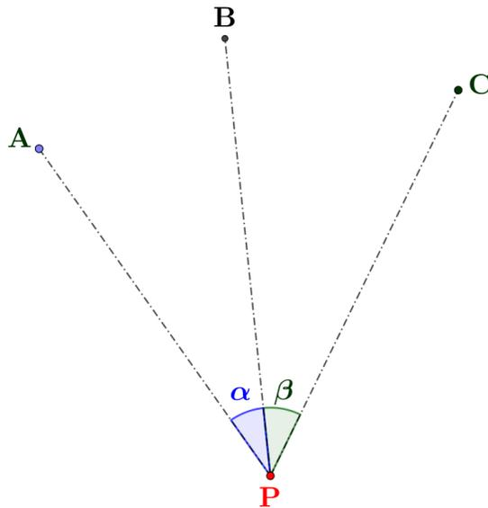
The points  $A$ ,  $B$ ,  $C$  and the angles  $\alpha$  and  $\beta$  are known. Determine the location of the observer point  $P$ .
