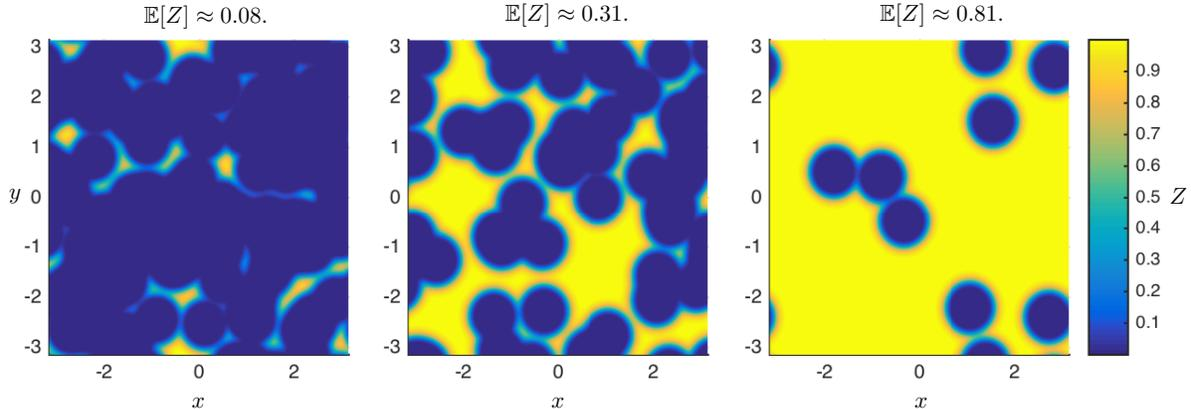
FIGURE 2: Surface plots of  $Z(x, y)$  for various bubble densities. Depending on whether regions of high or low  $Z$  percolate across the horizon determines whether we are in the metallic or insulating phase, as is clear upon comparing with Figure 1.
