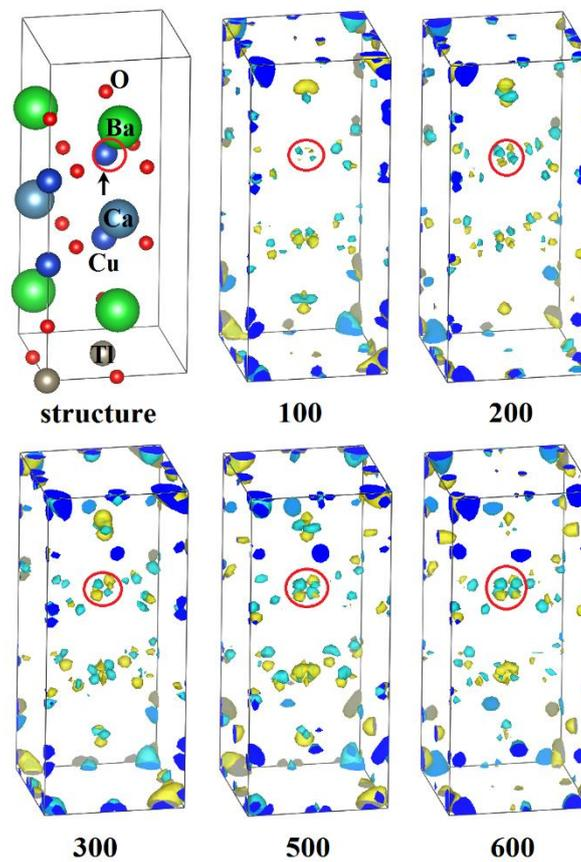
**Fig. 2** Crystal structure and the change of the electron cloud over time of  $\text{TlBa}_2\text{CaCu}_2\text{O}_7$ . The iso-surface is 0.05.
