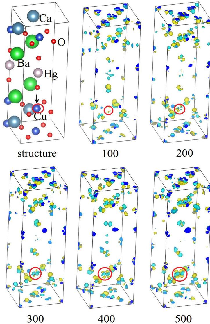
**Fig. 3** Crystal structure and the change of the electron cloud over time of  $\text{HgBa}_2\text{Ca}_2\text{Cu}_3\text{O}_8$ . The iso-surface is 0.05.
