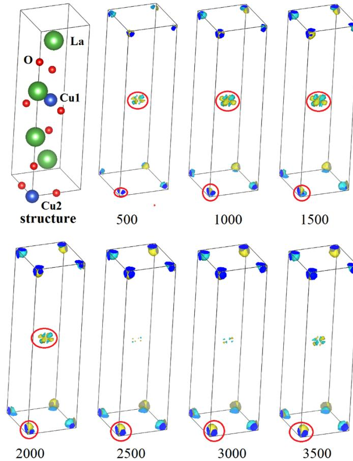
Fig.1 Crystal structure and the change of the electron cloud over time of  $\text{La}_2\text{CuO}_4$ . Plots were generated using VESTA <sup>[6]</sup>. The iso-surface is  $0.05 \text{ e/bohr}^3$ .
