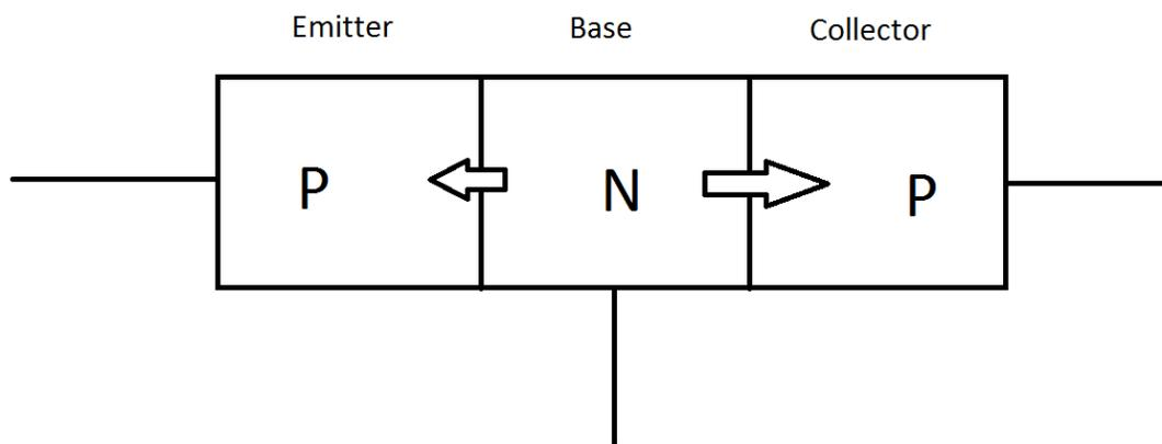
Figure 1: Schematic of a PNP bipolar junction transistor. As indicated by arrows, the collector-base barrier is larger than the emitter-base barrier.
