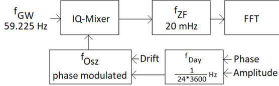
Figure 1): *Principle of the MSH method: The parameters for frequency drift and phase modulation of the auxiliary oscillator are iterated until the amplitude of the spectral line at  $f_{ZF}$  reaches a maximum.*
