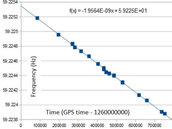
Figure 4): *Frequency  $f_{GW}$  of the Crab pulsar as a function of time. The dots are the initial frequencies of the 19 data strings (see table 2). Each stretches over a total duration of 97 hours. The start times were chosen so that the total duration contains as few data gaps as possible.*
