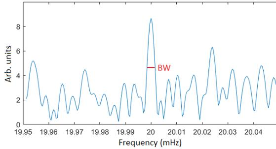
Figure 3): *The spectrum of the environment of the GW of the Crab pulsar after removal of the phase modulation by the MSH procedure and reduction of the frequency to 20 mHz. Source file = V1260445696, recording duration = 97 h. Only the narrow range BW is evaluated.*
