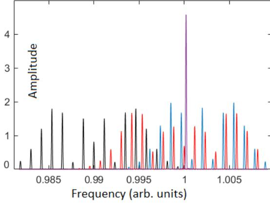
Figure 2): *Spectrum of a synthetic data set containing four GW with similar frequencies and the same energy. Three GWs are phase modulated in a 24-hour rhythm, one GW is unmodulated. The amplitude of this GW is higher by a factor of three because of the lack of splitting into 17 sideband frequencies. Noise and drift are missing because they would cause additional lines.*
