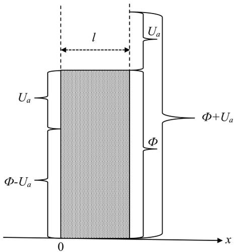
FIG. 6: Variation in height of barrier on both sides due to applied voltage.  $U_a$  denotes the variation in height of the barrier by an bias voltage.
