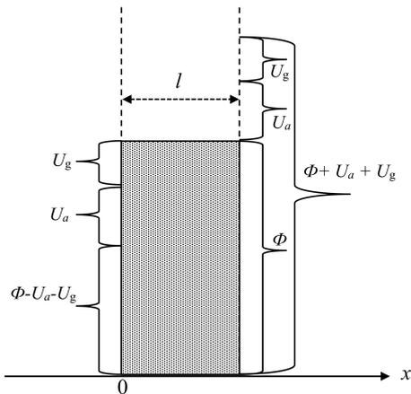
FIG. 7: Variation in barrier heights on both sides of the potential barrier due to applied voltage  $U_a$  and density gradient.  $U_g$  is the variation in barrier height due to the density gradient.
