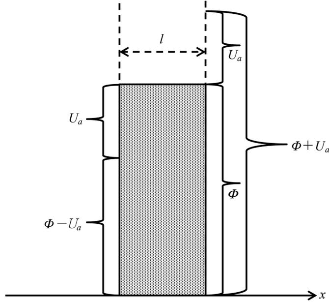
Figure 1: Variation in height of barrier in both sides due to applied voltage
