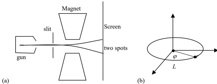
Fig.27 The Stern-Gerlach experiment apparatus.
