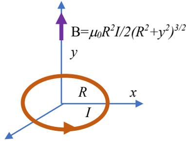
Fig.24 The magnetic field of a single coil.
