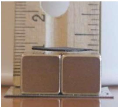
**Fig 3:** Pyrolytic carbon levitating above a strong magnet (Image credit scitoys.com )
