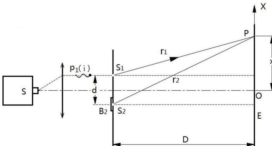
Fig. 3.3A Single photon double-slit interference ( $S_2$  blocked)
