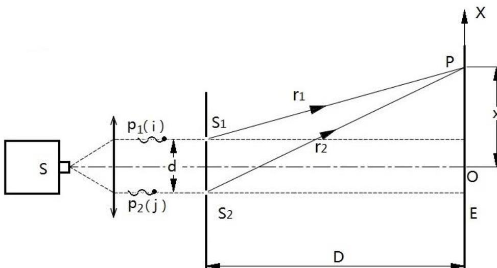
Fig. 3.2 Single photon double-slit interference
