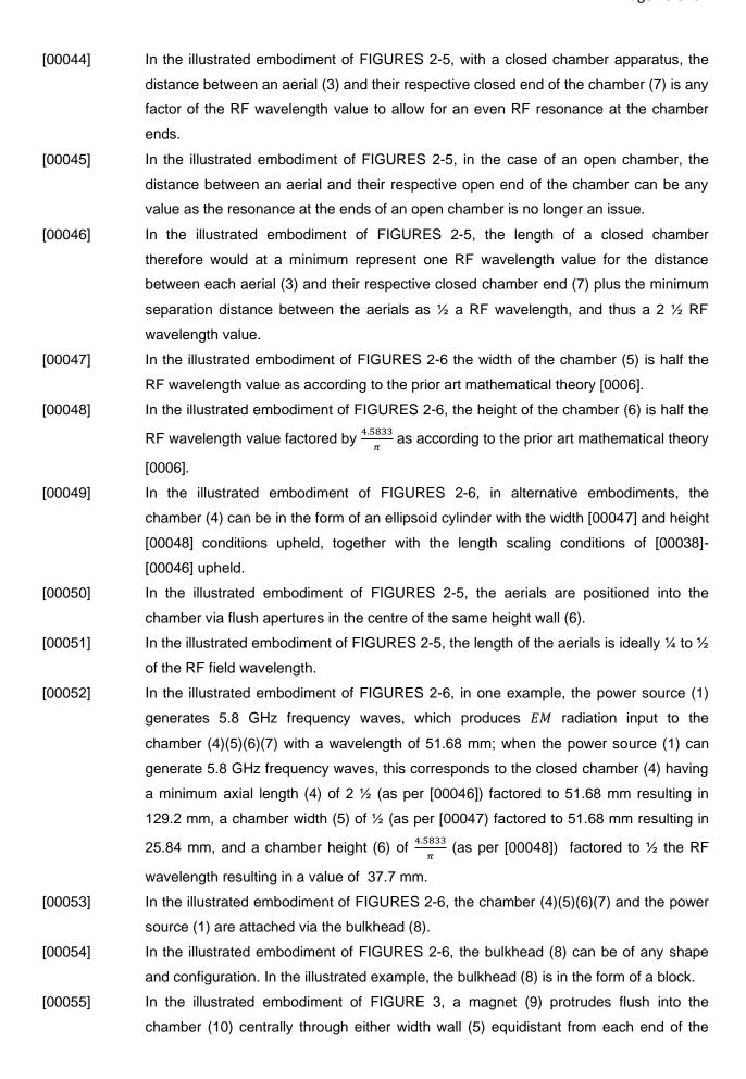
chamber (7) and thus equidistant from each of the aerials (3), although varying locations maybe be used for the position of the magnet protruding flush into the chamber between the aerials in either of the width (5) or height (6) walls.
