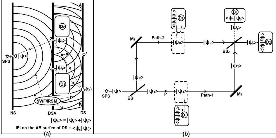
FIG. 2. Schematic diagrams of Young's Double-Slit and Mach-Zehnder Interferometer
