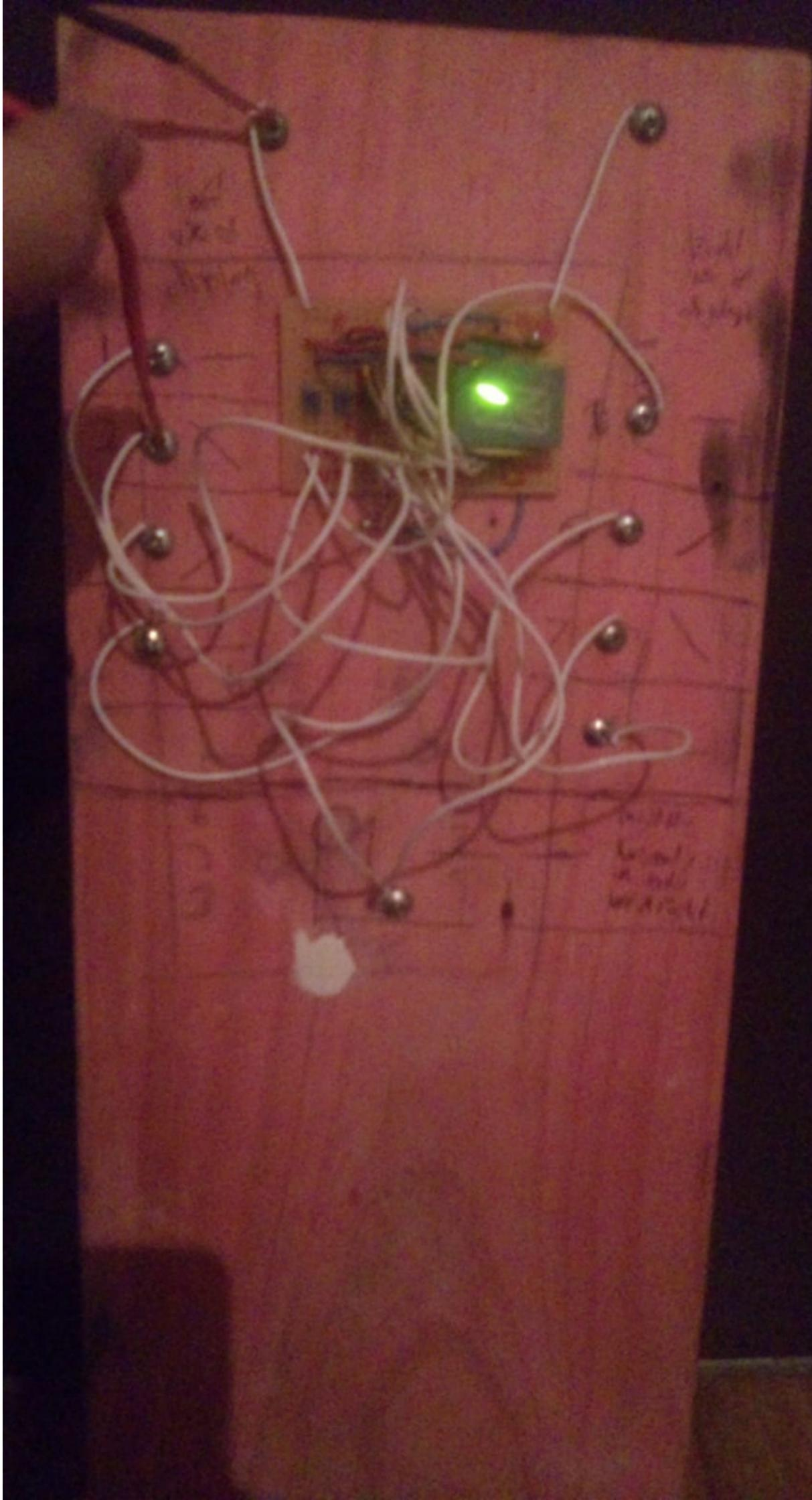
Testing screw 3 (negative on ground, positive on screw 3):
