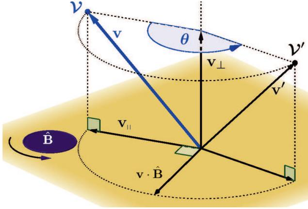
Figure 2: Relations between vector  $\mathbf{v}$ ; its components perpendicular and parallel to  $\hat{\mathbf{B}}$ ; and the rotated vector  $\mathbf{v}'$ .
