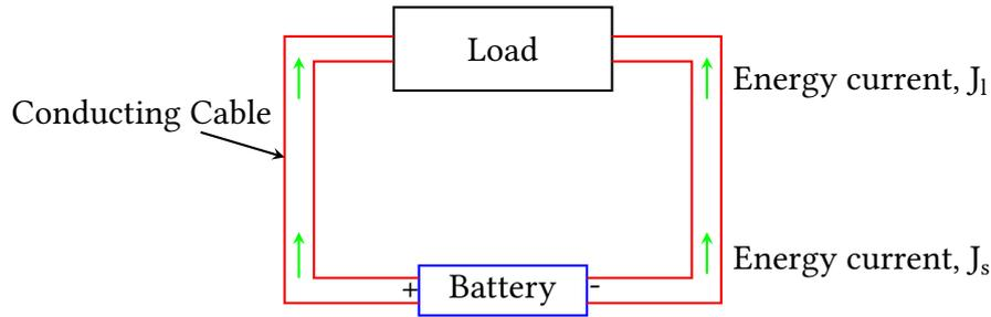
FIGURE 1. Battery supplying power; energy current flows within the conductor from both battery terminals. Current  $J_s$  leaves source,  $J_l$  enters load. Energy current direction is independent of electric current direction.
