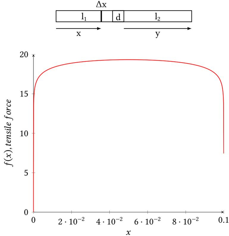
FIGURE 6. Graph showing variation of Ampere tensile force in a long conductor with current  $I$ .  $f(x)=\ln(0.1-x)-\ln(0.1 \times 10^{-10})+\ln(x+10^{-10})$ . For  $I=1000\text{A}$ ,  $l=0.1\text{m}$ ,  $d=1 \times 10^{-10}\text{m}$ , the maximum force at the middle is  $1.93\text{N}$ .
