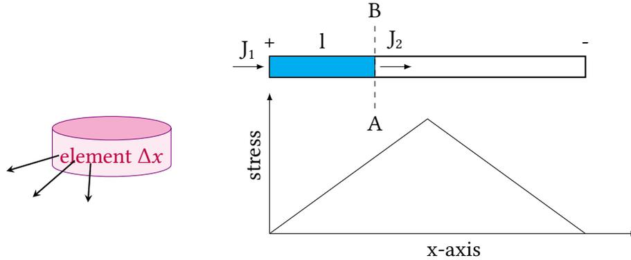
FIGURE 2. Left: A typical  $\Delta x$  element of a conductor wire of circular cross section; the radiation intensity is symmetrical and points in the normal direction to the surface. Right: A long conductor with electric current  $I$ ; a section of length  $l$  from left terminal, resistance  $R$ . The graph shows the variation of compressive stress on an element of length  $dl$  of the conductor at various distances within the conductor.
