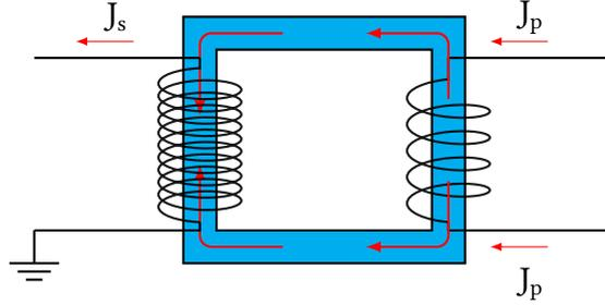
FIGURE 5. Delta-wye ( $\Delta$ -Y) step-up transformer action. The right primary winding is connected to the armature winding through a 3-phase delta connection. The left secondary winding connects to the transmission cables through a wye connection. Energy current  $J_p$  jumps the air gap entering the iron towards the secondary and jumps the air gap into the winding giving the secondary energy current  $J_s$ .
