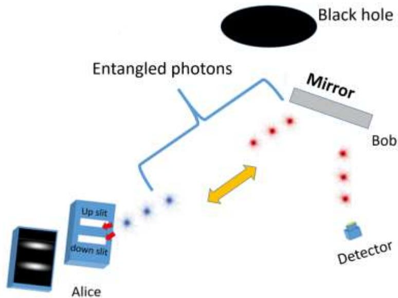
Figure 1: Entangled photons traveling in two opposite directions towards Alice and Bob. The photons travelling to the left will pass through a double slit setup and will be detected on Alice screen. As long as Bob tilts the mirror in the direction that will reflect the entangled photons travelling to the right to a position detector, Alice will see a non-interference pattern on her screen.
