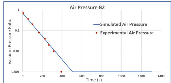
Figure 3: Our setup required about 300 seconds to get to a vacuum quality sufficient to neutralize the Bournoulli effect.
