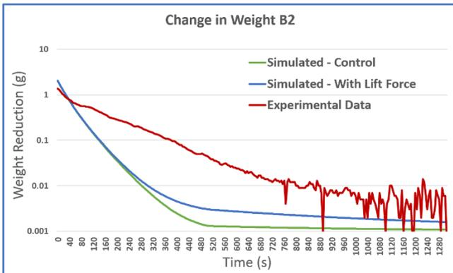
Figure 4: Experimental data showing reduction in measured mass.
