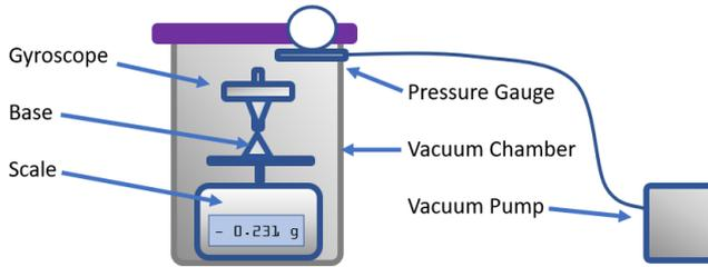
Figure 1: Experimental setup with a gyroscope on a sensitive scale, in a high quality vacuum.
