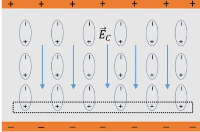
Fig. 3. The polarization of the atoms in a dielectric material due to the irrotational electric field from electric charges.
