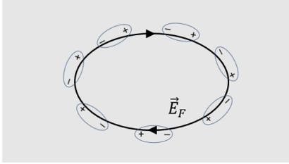
Fig. 4. The polarization of the atoms in a dielectric material due to the rotational electric field, generated by a time-varying magnetic-flux density  $\vec{B}$  in Faraday's law.
