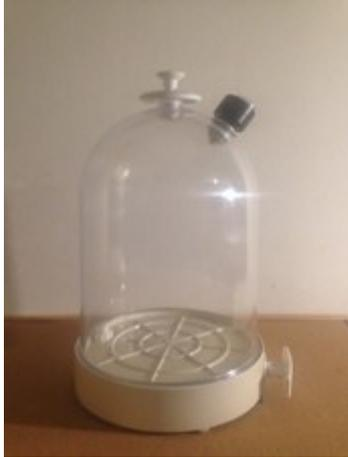
**Figure 1.** Vacuum chamber with integrated hand pump
