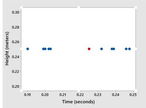
**Figure 2.** Path-time diagram. Free fall of the metal disk. The red dot represents the nominal value according to Galileo Galilei's law of falling bodies. The blue dots represent the measured values.
