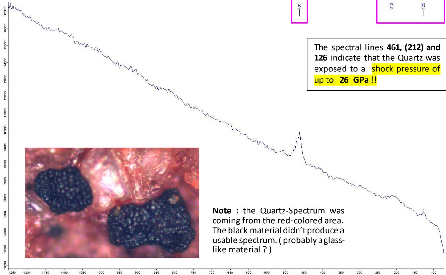
**Note** : the Quartz-Spectrum was coming from the red-colored area. The black material didn't produce a usable spectrum. ( probably a glass-like material ? )
