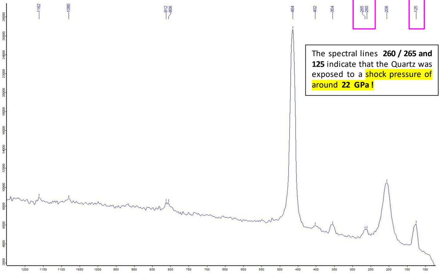
The spectral lines **260 / 265** and **125** indicate that the Quartz was exposed to a **shock pressure of around 22 GPa !**
