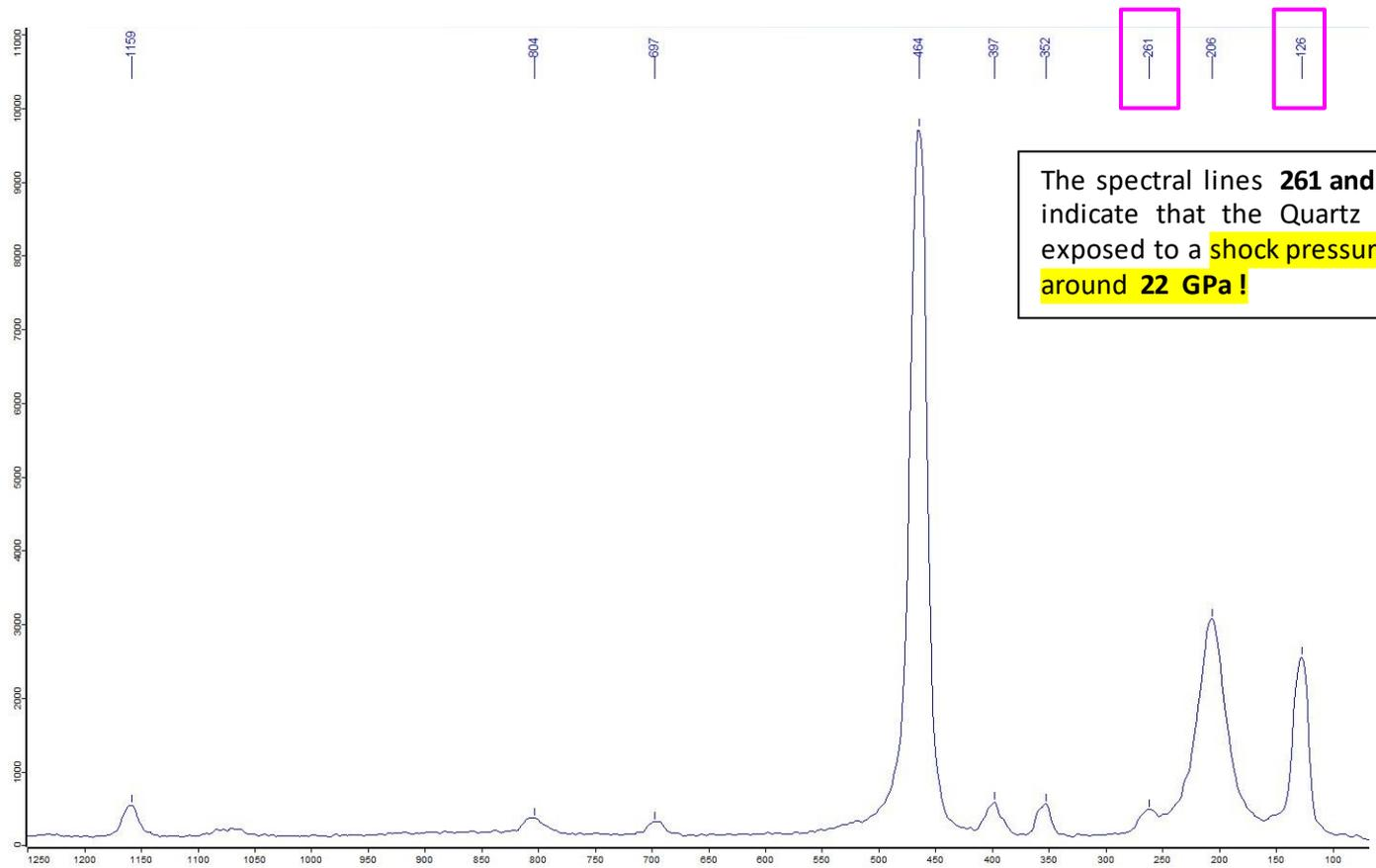
The spectral lines **261** and **126** indicate that the Quartz was exposed to a **shock pressure of around 22 GPa!**
