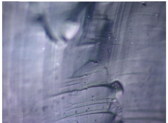
Sample Site **23**: Stone 1\_spectra 1 indicates: **Quartz + (Orthoclase)**
