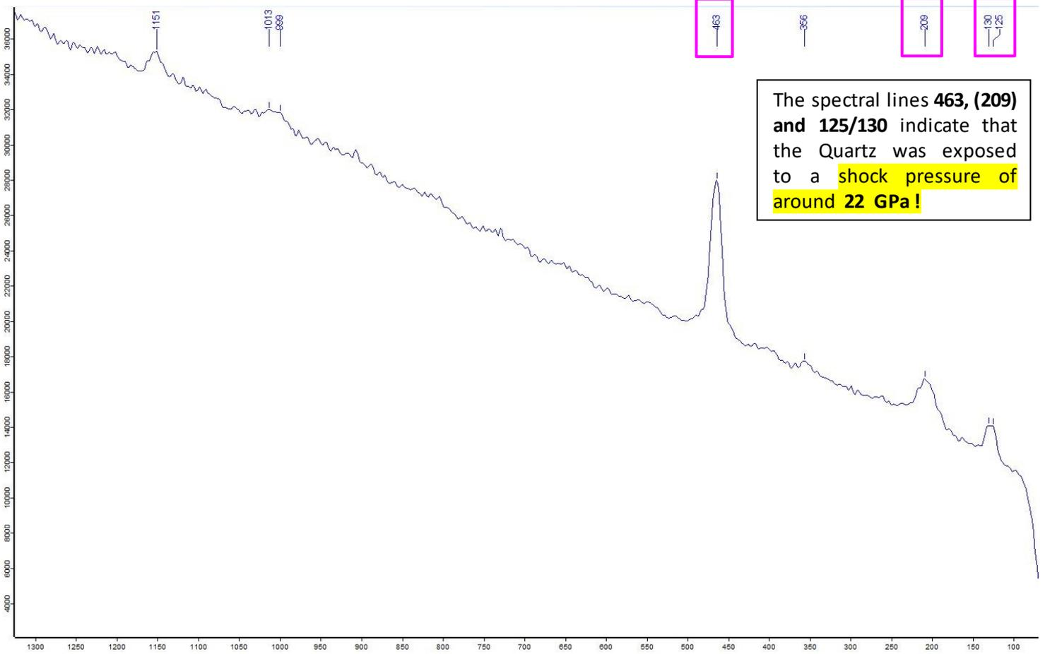
The spectral lines **463**, **(209)** and **125/130** indicate that the Quartz was exposed to a **shock pressure of around 22 GPa !**
