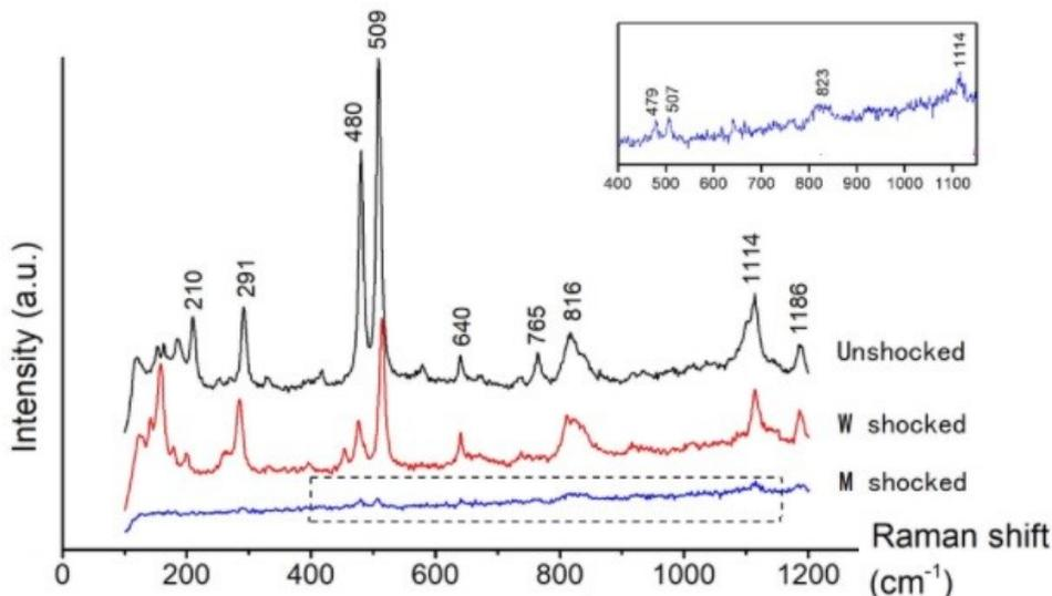
Weakly shocked alkali feldspar mainly developed irregular fractures and undulatory extinction. Note that the Raman-lines 210 and 765 are missing in the w-shocked feldspar, and an additional line at ≈ 150 appears.
