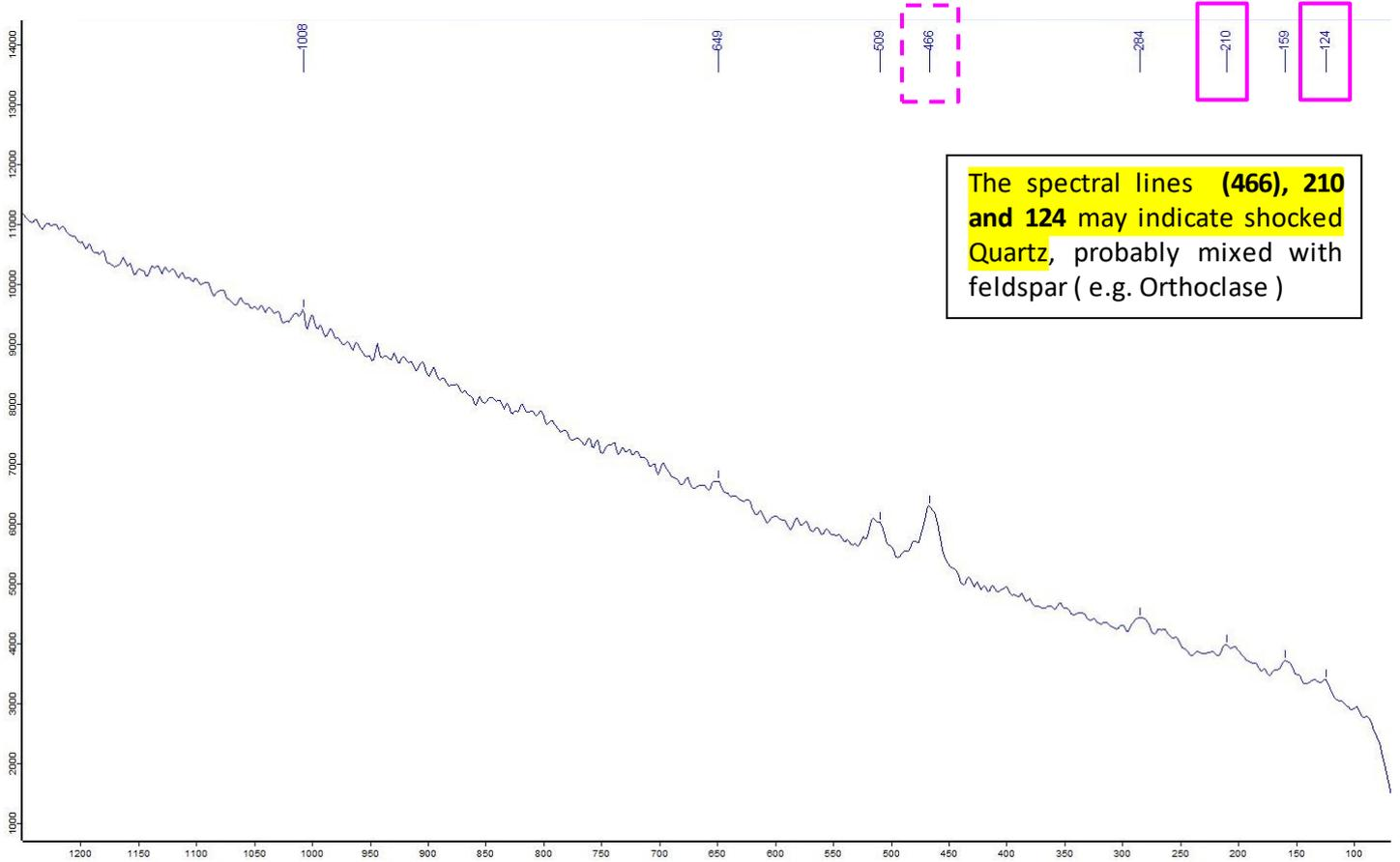
The spectral lines **(466), 210 and 124** may indicate shocked Quartz, probably mixed with feldspar ( e.g. Orthoclase )
