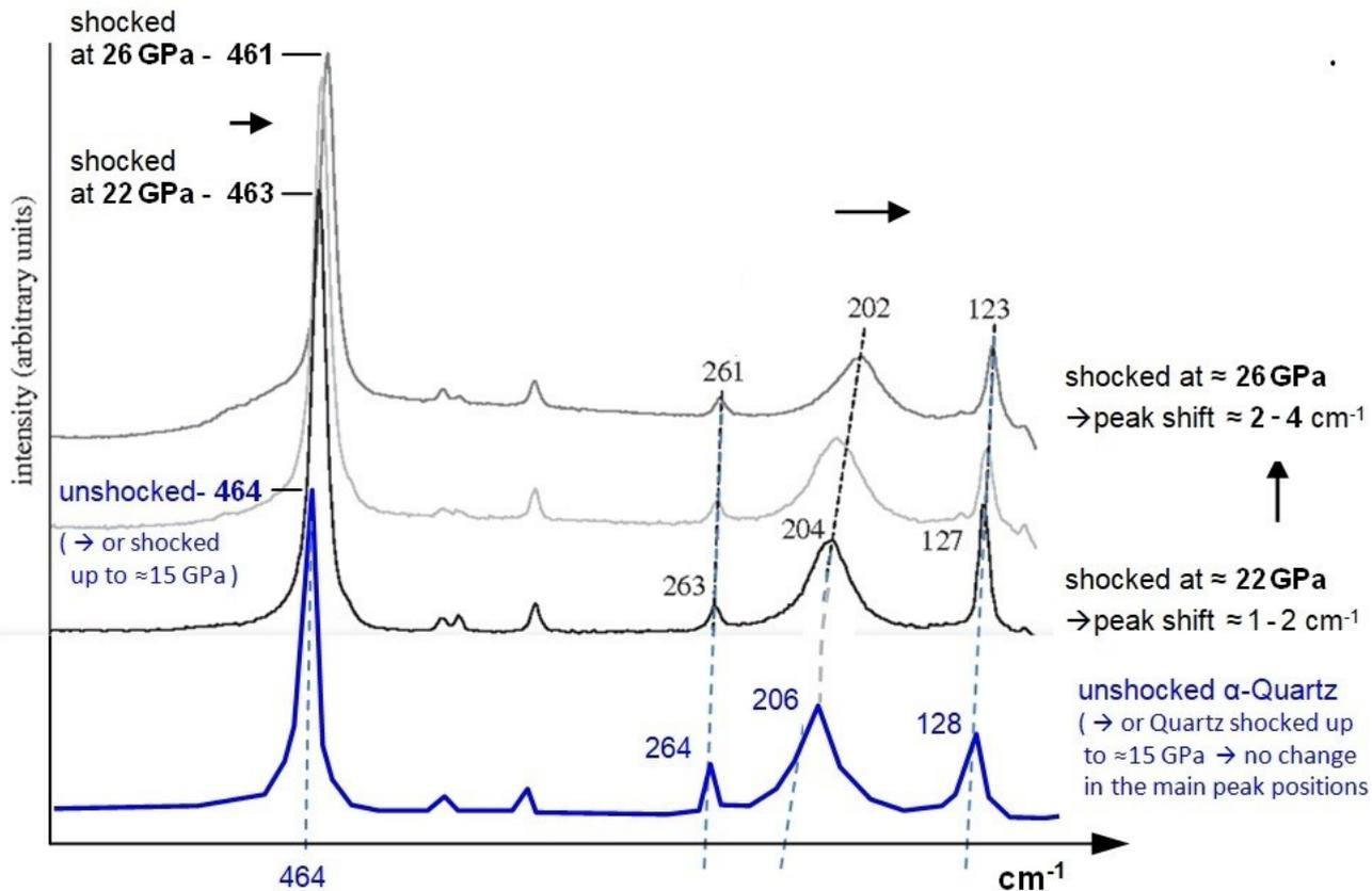
Quartz shocked with 22 GPa and 26 GPa shows shifts of the main RAMAN-peaks of 1 - 4 cm<sup>-1</sup> to lower frequencies
