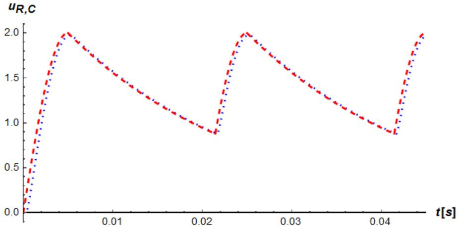
Figure 6: Graph of the piecewise linear diode model, ideal (red), piecewise linear (blue),  $\frac{R}{r_f} = 10$
