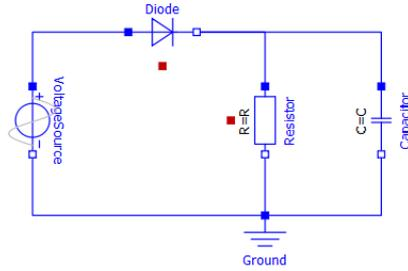
Figure 3: To reduce the magnitude of the ripple voltage a capacitor  $C$  is added in parallel to the load resistor  $R$  of the basic circuit shown in Figure 1.
