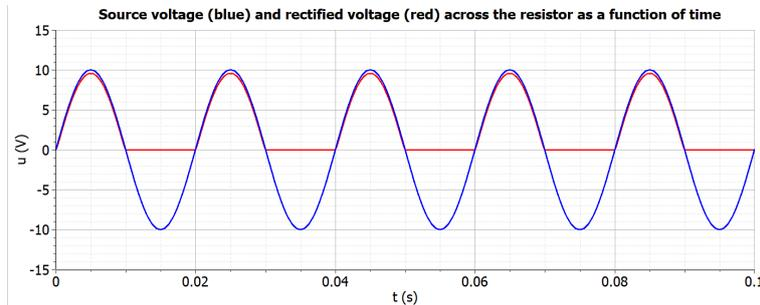
Figure 2: Graph of the rectified voltage  $u_R(t) = u_{ripple}$  measured over the load resistor  $R$  of the circuit displayed in Figure 1.
