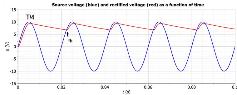
Figure 4: Graph of the decreased magnitude of the ripple voltage due to having added a capacitor  $C$  in parallel to the load resistor  $R$ . In red is depicted the source signal  $u_s(t)$  and in blue the voltage  $u_{R,C}(t)$ . The time  $t_{fb}$  at which the diode becomes forward biased during the second cycle is shown as well. The time difference  $\Delta t = t_{fb} - T/4$  marks the period of the diode being reverse biased during which the loaded capacitor discharges.
