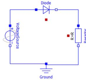
Figure 1: Graph of the most basic rectifying circuit consisting of a harmonic voltage source, a diode and an ohmic resistor only.
