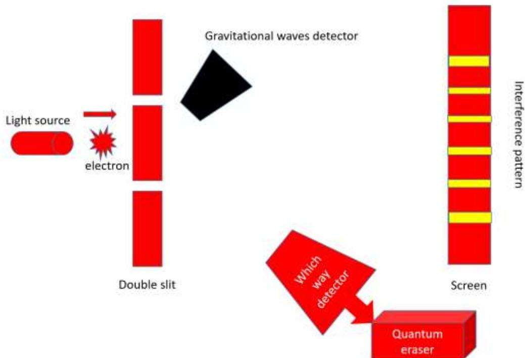
Figure 2: The second group of electrons that is first passing phase A (the which-path detector) and then passing through phase B (the quantum eraser). The gravitational waves detector measures the gravitation waves just after phase A and before phase B. This second group generates an interference pattern on the screen (peaks and valleys).
