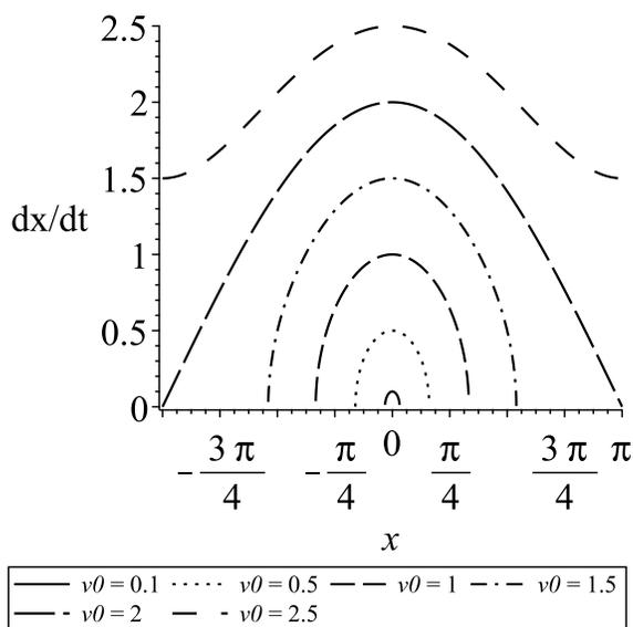
Figure 5: Exact phase space diagram of the pendulum
