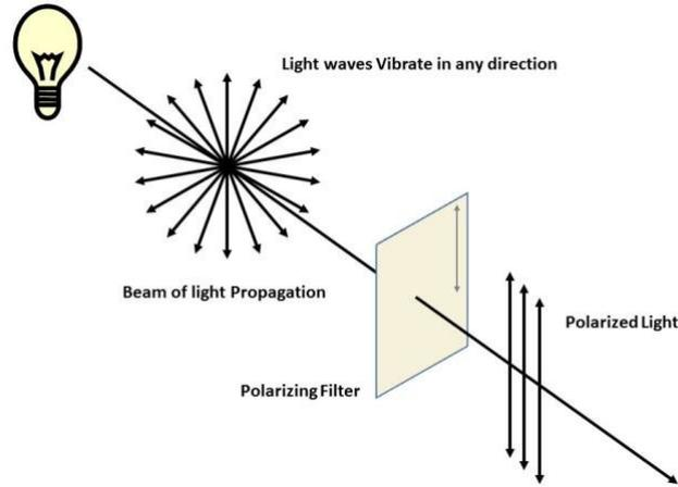
Figure 2: Light source producing unpolarized light which passes through a polarizer to produce a polarized light wave. Web Reference: [https://www.researchgate.net/publication/328100369\\_Polarised\\_infrared\\_light\\_enables\\_enhancement\\_of\\_histo-morphological\\_diagnosis\\_of\\_prostate\\_cancer](https://www.researchgate.net/publication/328100369_Polarised_infrared_light_enables_enhancement_of_histo-morphological_diagnosis_of_prostate_cancer)
