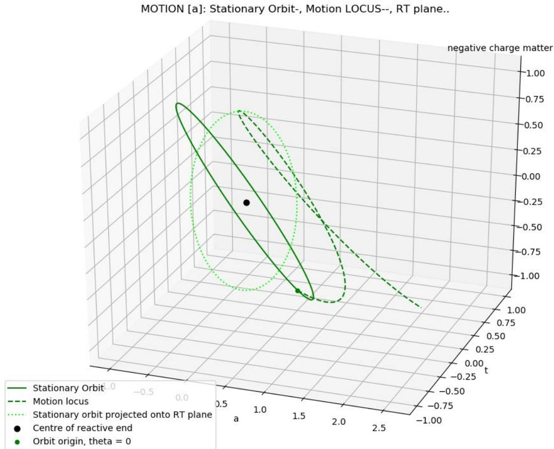
*Figure 8: Motion of the reactive end over one energisation cycle, showing the spiral nature of the movement, for an electron with  $\tau = 0.5$  and  $R_{RE} = 1$ . Vertical axis is  $[r]$ . Note that the helix angle is not constant, but rather is a periodic variable.*
