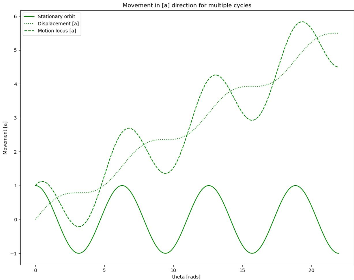
*Figure 7: Cumulative displacement in the [a] direction over multiple energisation cycles, for an electron with  $\tau = 0.5$  and  $R_{RE} = 1$ .*
