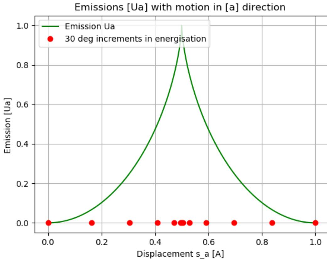
*Figure 4: Emissions in [a] as a function of displacement in the same direction. Displacement has been normalised by dividing by  $P_a = \tau\pi$ . Red dots indicate sample locations of the reactive end, and show how it initially moves quickly, slows to a momentary stop, and then quickens its displacement again.*
