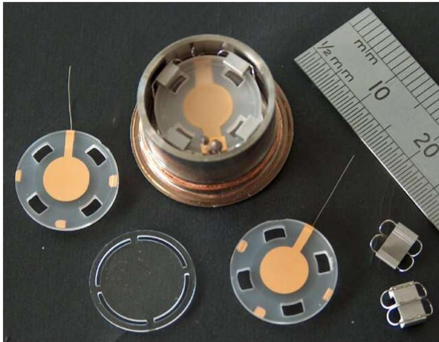
“The new detector designed by the research team at the CDM to pick up high frequency gravitational waves
