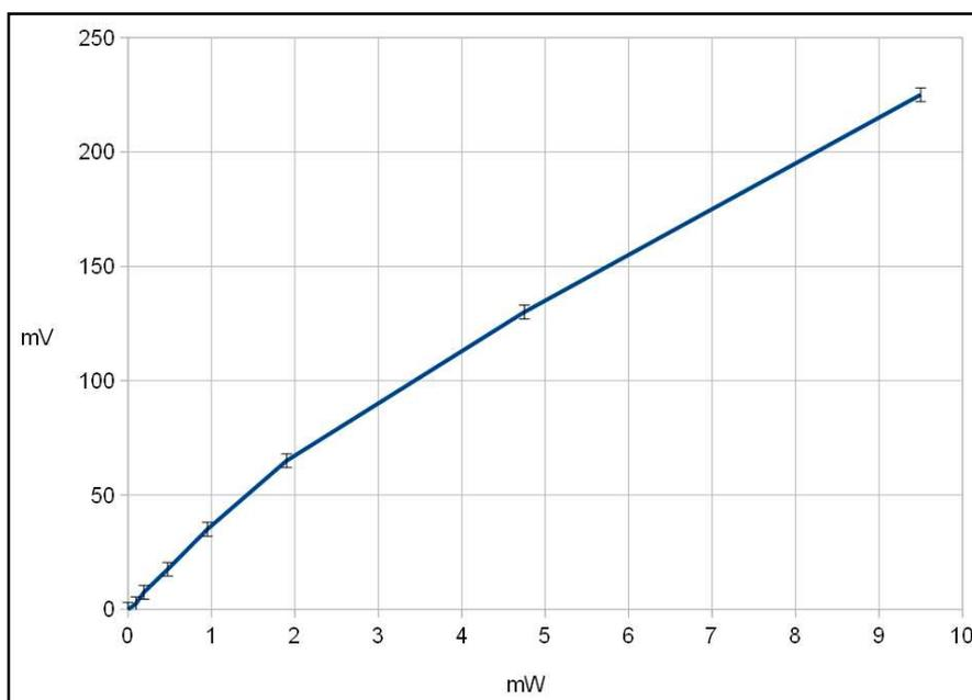
**Fig. 4: Lock-in-amp output vs. light power through the sound hole**
