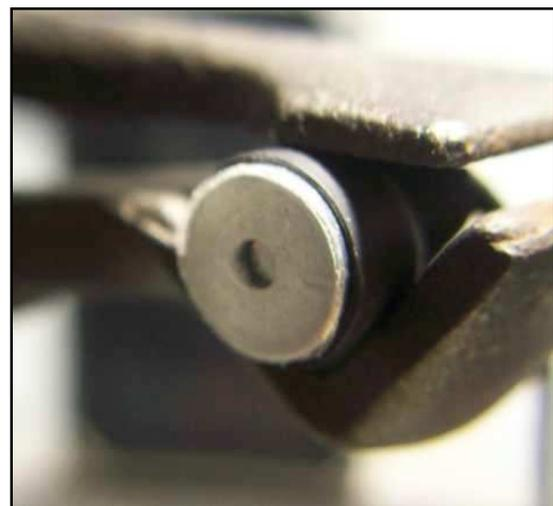
**Fig. 2 : Electret microphone**
