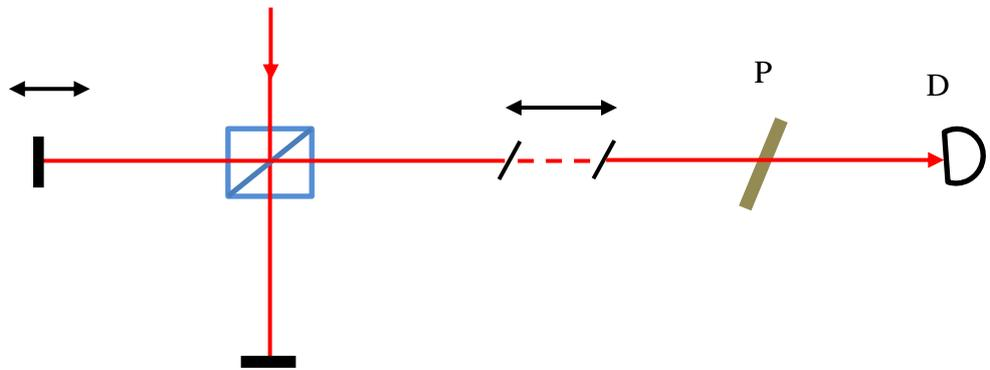
Figure 2. Simplified scheme of experiment with Michelson interferometer.
