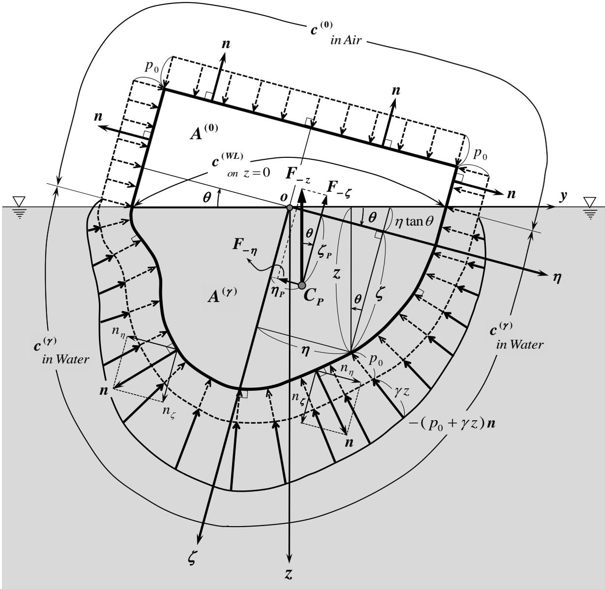
Fig. 2 Hydrostatic pressure and center of pressure acting on the inclined floating body with arbitrary form.
