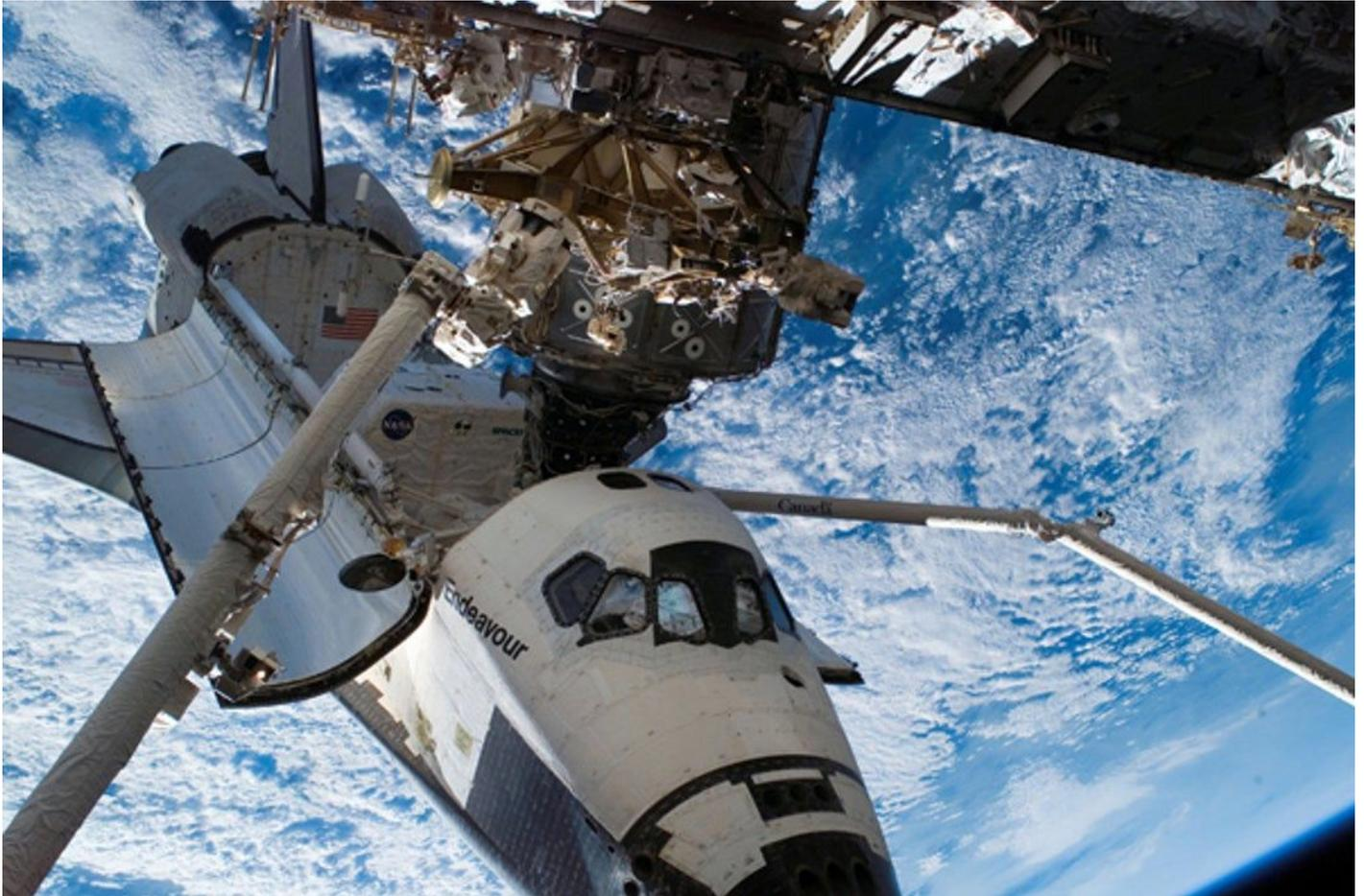
(Canadian Robotic arm of Space Shuttle. Courtesy: <https://www.cnet.com/pictures/canadarm-the-zero-gravity-grappler-pictures/2/>)
