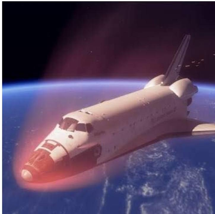
(Atmospheric Heating & Reentry. Courtesy: NASA)
