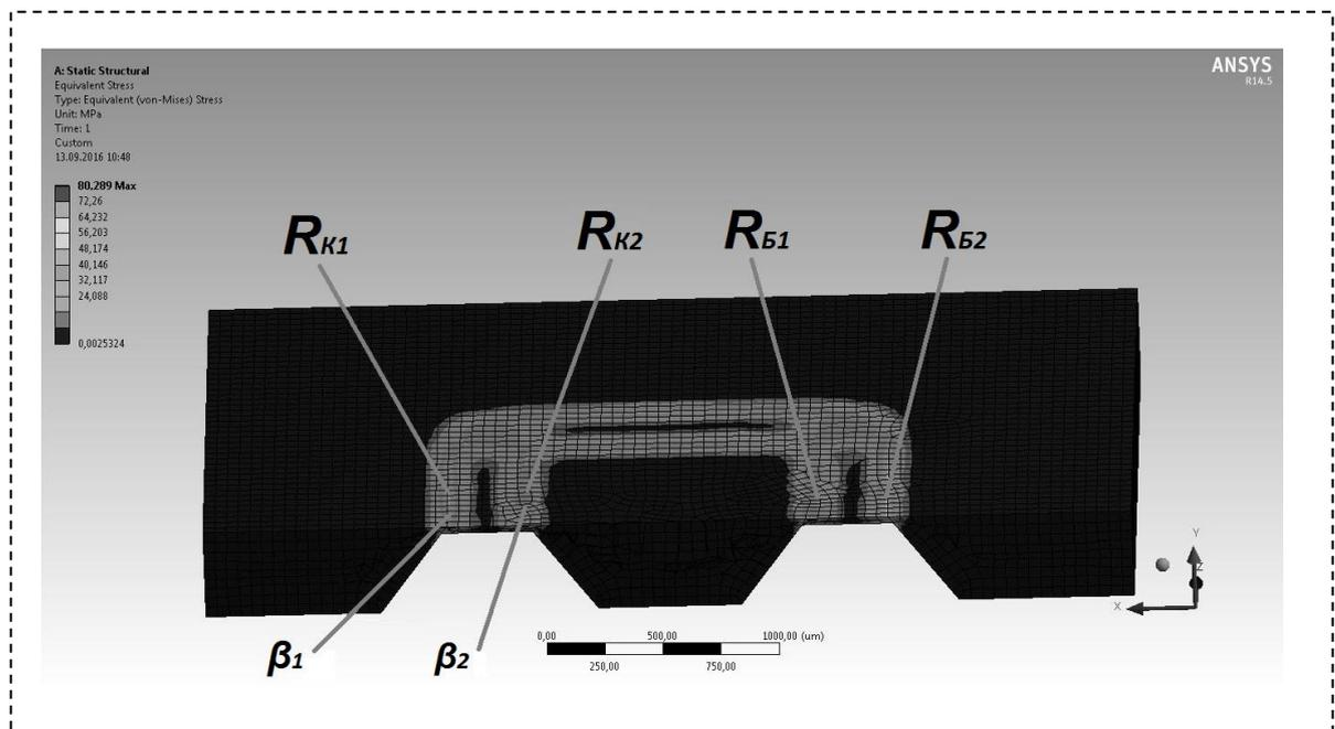
Fig. 3. Mechanical stresses of silicon membrane and the arrangement of strain elements on die
