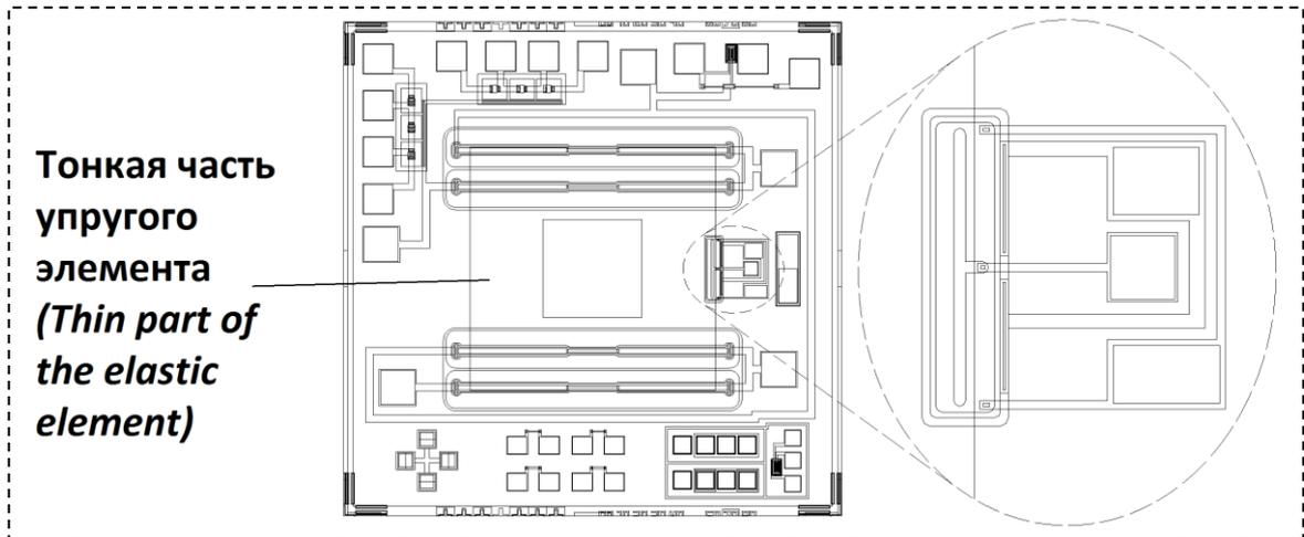
Fig. 2. Die with electrical circuits of Wheatstone bridge and with separately formed BTT
