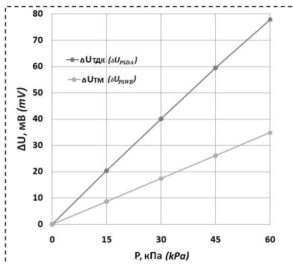
Fig. 7. Linear dependence of output signal by pressure
