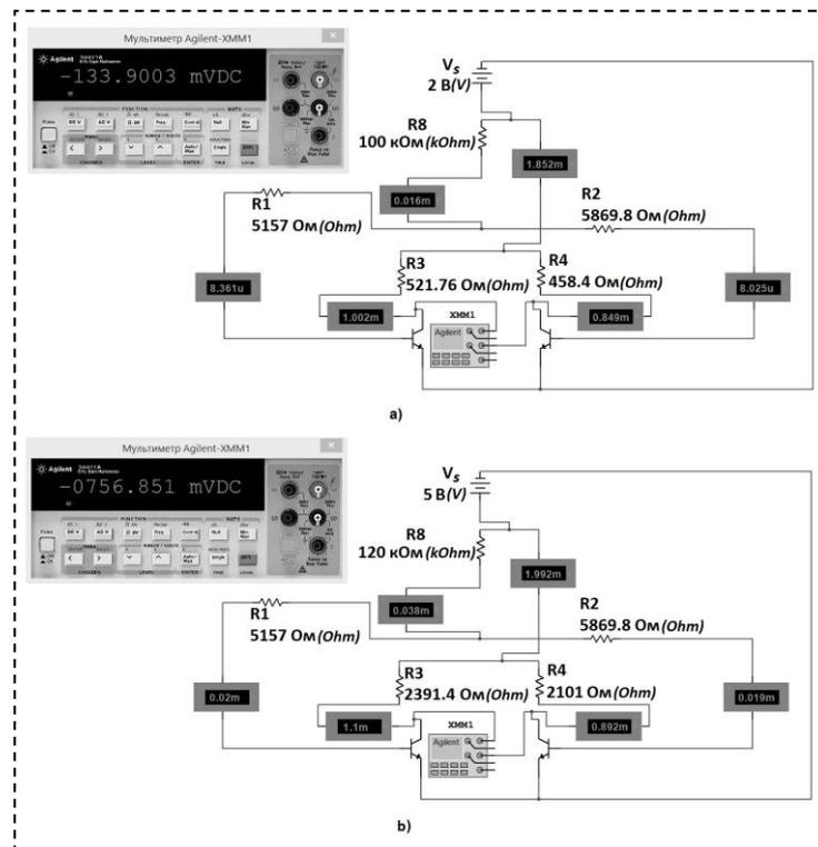
Fig. 9. Modeling of circuit for: a) samples obtained in practice, b) samples with changed values of elements
