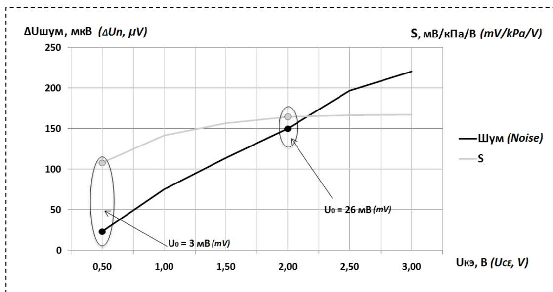
Fig 8. Dependences of noise's component from output signal and the sensitivity by voltage  $U_{\text{CE}}$
