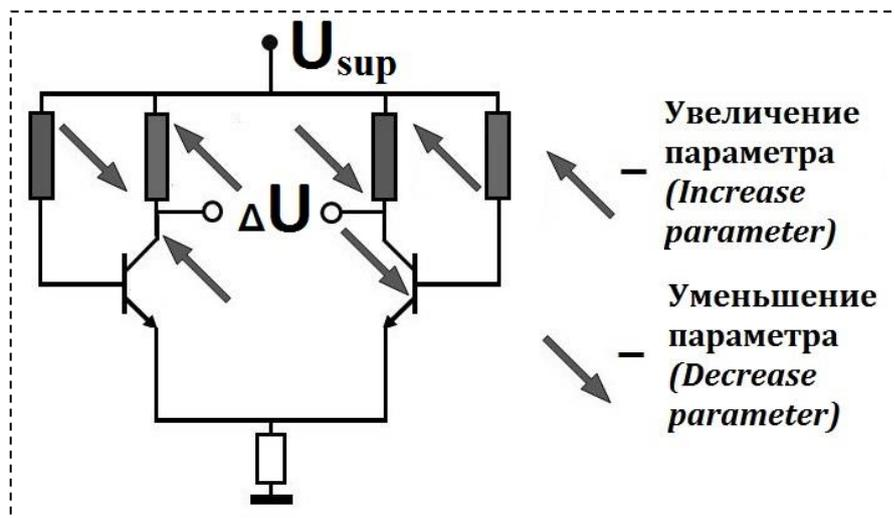
Fig. 1. Die with electrical circuits of differential amplifier
