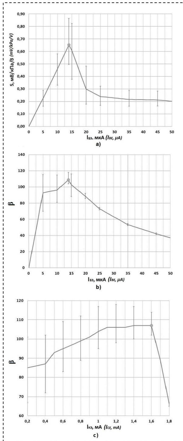
Fig. 5. Dependencies: a) sensitivity  $S$  by current of basic's circuit  $I_{\text{BE}}$ , b) gain  $\beta$  by current of basic's circuit  $I_{\text{BE}}$ , c) gain  $\beta$  by current of collector's circuit  $I_{\text{CE}}$
