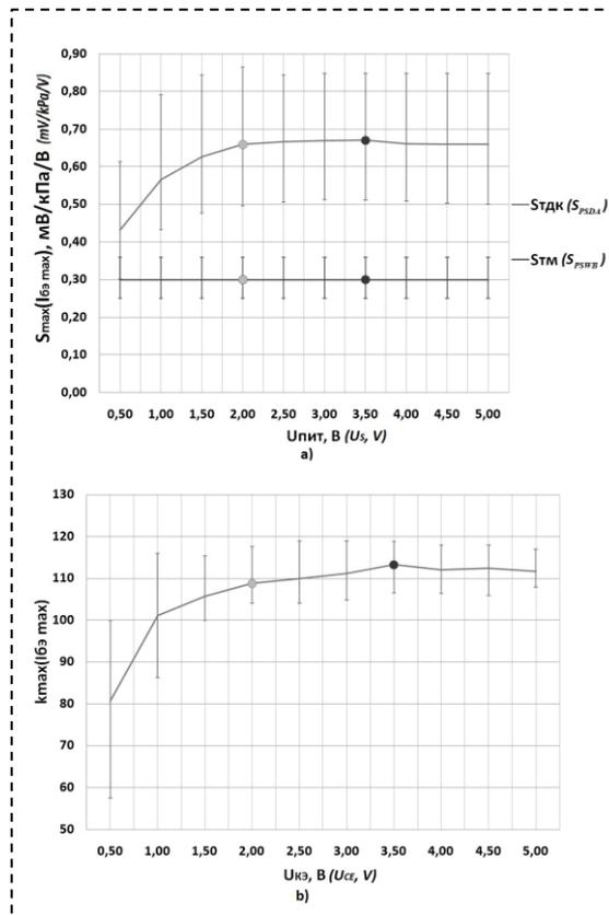
Fig. 6. Dependencies: a) sensitivity  $S$  by voltage of base's circuit  $U_{CE}$ , b) gain  $\beta$  by voltage of base's circuit  $U_{CE}$
