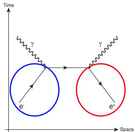
**Fig. 4.** A Feynman diagram showing the mutual annihilation of a bound state electron-positron pair into two photons. The electrons and positrons were regarded as counter-rotating phasors for the purpose of followed discussion. Image source: [4]
