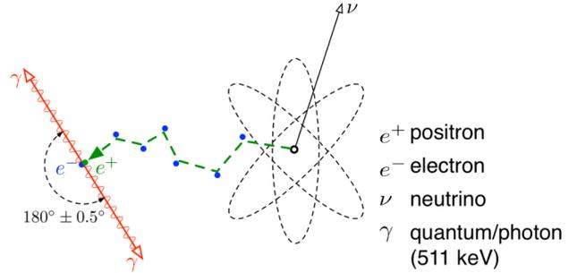
**Fig. 1.** Naturally occurring electron-positron annihilation as a result of beta plus decay. Image source: [4]
