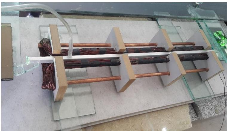
Fig. 6: Longitudinal electrical magnet with two parallel rows of a coiled wire
