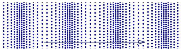
Fig. 5: Light as a longitudinal wave similar to a sound wave
