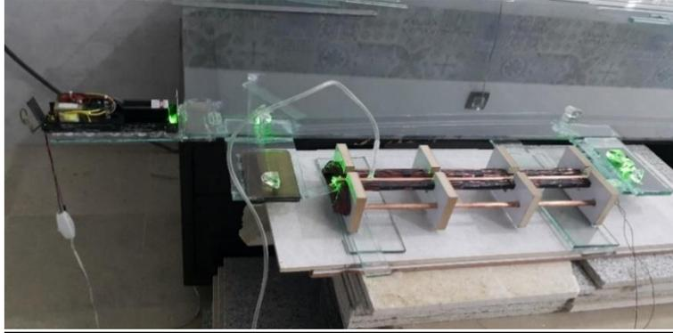
Fig. 7: Experimental apparatus setup with horizontal electrical magnet
