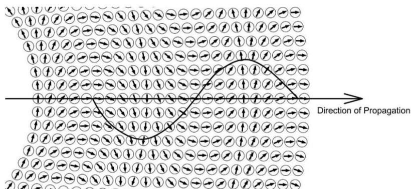
Fig. 11: Model of fluctuating and propagation of radio waves in space
