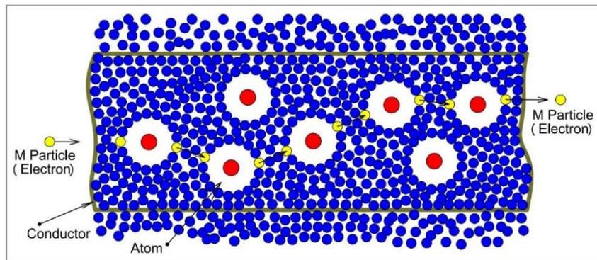
Fig. 13: Electrical current flow through a conductor
