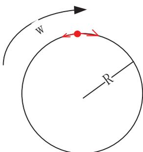
Fiber optic gyroscope has been widely used, and its working principle can be well explained by classical Newtonian mechanics. The speed of the fiber optic gyroscope relative to the ring is as follows: assuming that the speed of light in the ring is  $C_0$  when the fiber optic ring is stationary.
