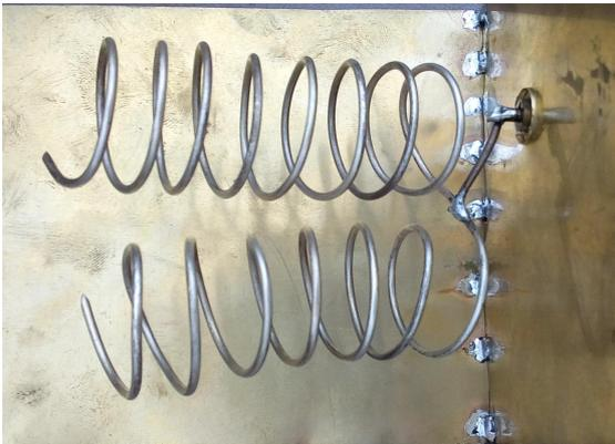
Figure 2: Double helix in front of the  $90^\circ$  reflector. On the right you can see the backside of the coax socket. The 20 mm short piece of wire to the helix simplifies the electrical matching (see text). For continuous operation a mechanical fixation of the helix is recommended to avoid a short circuit with the reflector.
