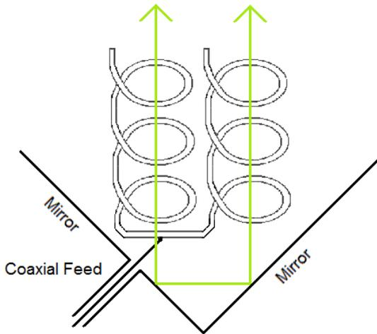
Figure 1: The angle mirror deflects every wave coming from above by exactly  $180^\circ$ . This also applies to waves arriving at an angle. Only on the short horizontal path below the helix the polarization sense is inverted.
