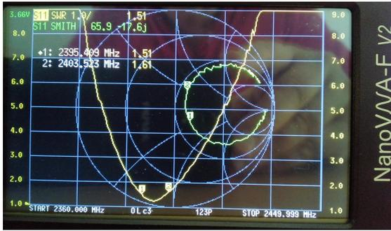
Figure 3: Display of the VNA. At resonance (2401 MHz), the SWR is less than 1.3 (yellow U-curve). The green circle shows how much the reactance changes as a function of frequency.
