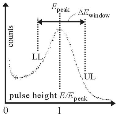
Figure 1. PMT pulse-height response
